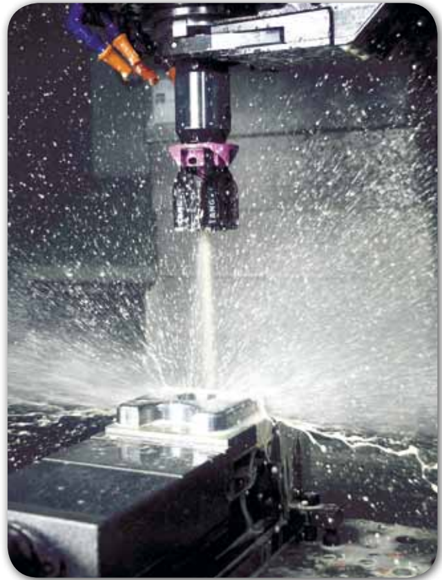
Rinse work pieces and fixtures by using internal coolant with the spindle stopped.
