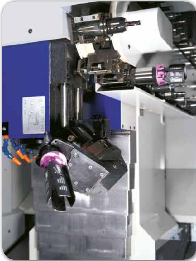
Exchange automatically from tool magazine.
