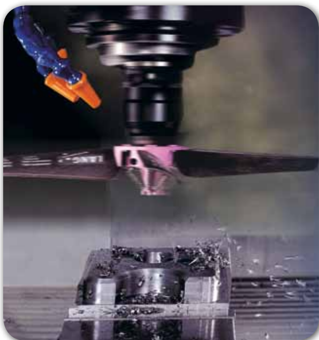
Move the rotating Clean•Tec up to 100-150 mm clearance above the work piece at 3-10 m/min. feed.
